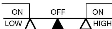
Figure 4-6 Dev. Band Breakaway Alarm [Hold On = Yes] (Alarm Code 03, Alarm release in the first alarming situation)
