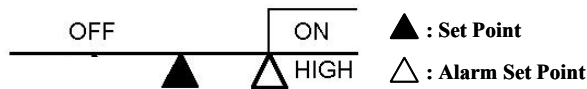
Figure 4-2 Upper Limit Deviation Alarm [Hold On = Yes] (Alarm Code 01, Alarm release in the first alarming situation)
